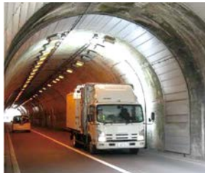
*A moving vehicle performs laser scanning to automatically measure tunnel deformation.
