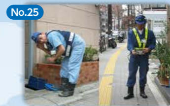
No.25 無収水削減技術 (漏水調査) Technology for Non-Revenue Water Reduction (Leakage Investigation)
