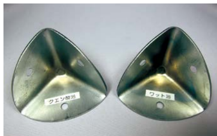
Left: Citric acid bath undercoat (little color irregularities) Right: Conventional bath undercoat (significant color irregularities)
