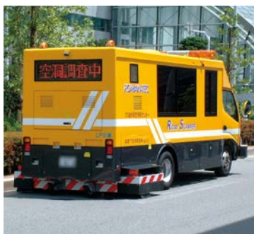
Radar survey for subsurface void detection
