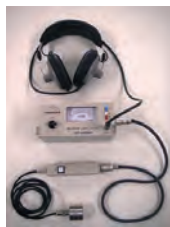
Leakage test using an electronic detector ※ 4
